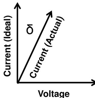
Figure III: Loss Tangent for Practical Capacitor
